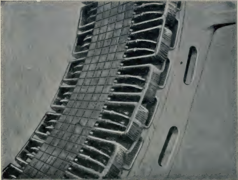
FIG. 258.—Stator Winding with similarly shaped Coils.
